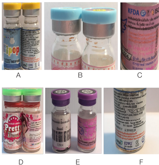
Figure 2 : External product defects [A: dirty products; B: abnormal stain around bottleneck; C: unclear/unreadable label; D: scratched label; E: application of other labels that obscure text; F: expired product]
