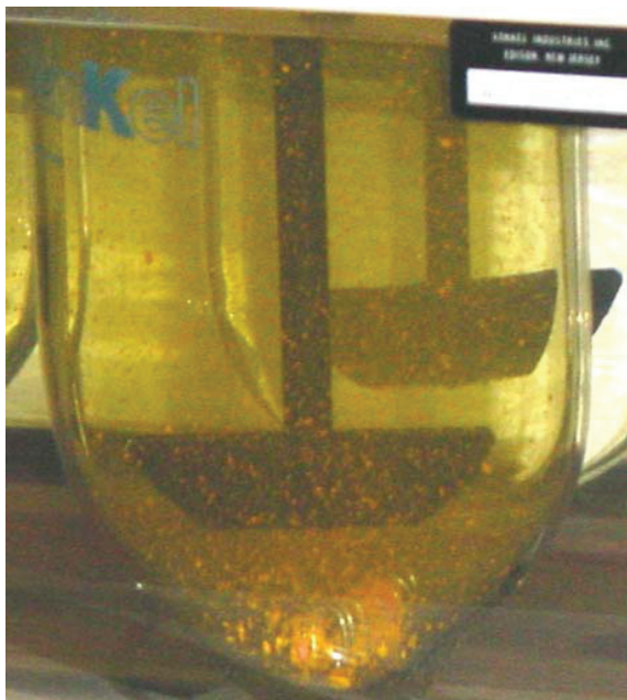
Fig. 3 Particles from contents of Turmeric capsules centered under the paddle in cone-shaped piles.
